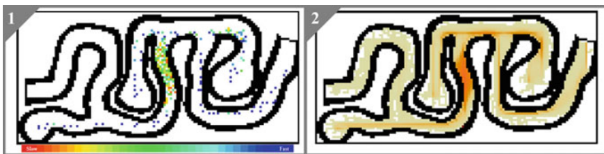
Fig. 3.12 Screenshots of the CZ user interface: 1 Instantaneous velocity of each agent is dynamically displayed. In the middle section local velocities are clearly lower due to congestion. 2 Dynamically displayed corresponding HM confirms the over-crowding of the middle section of the plan
