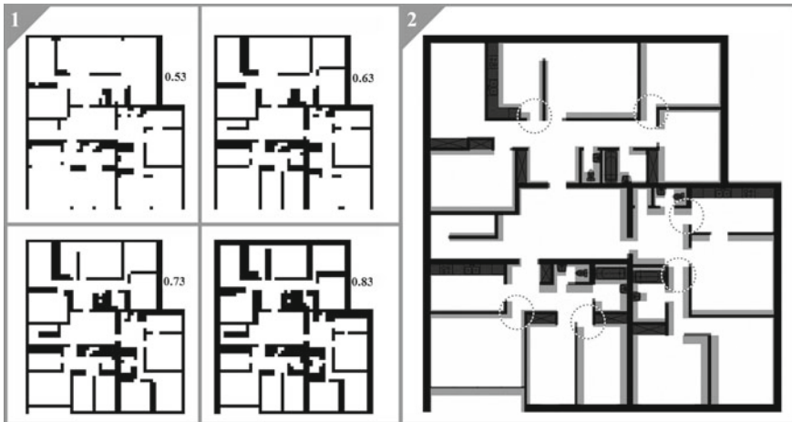
Fig. 3.19 1 The quality of binarized floor-plan is sensitive to the value of threshold t . 2 Binarization at t = 0.73 produces the best detail. For comparison the result is shown as semi-transparent with the original floor-plan shown in black. Circles indicate overly narrow parts of corridors and door openings which require “manual” alterations
