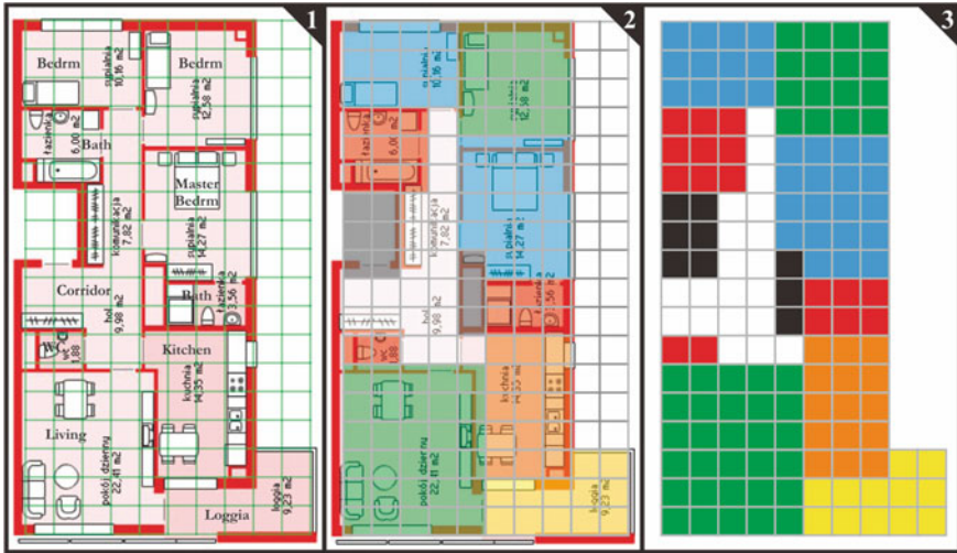
Fig. 1.4 A single apartment in a typical upper-income high-rise MFRB. Convention as in Fig. 1.2, grid size: 0.93 m
