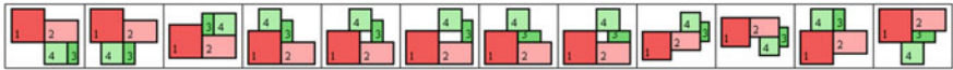
Fig. 1.12 The algorithm produced many poor layouts due to uncontrolled relative distances among rooms
