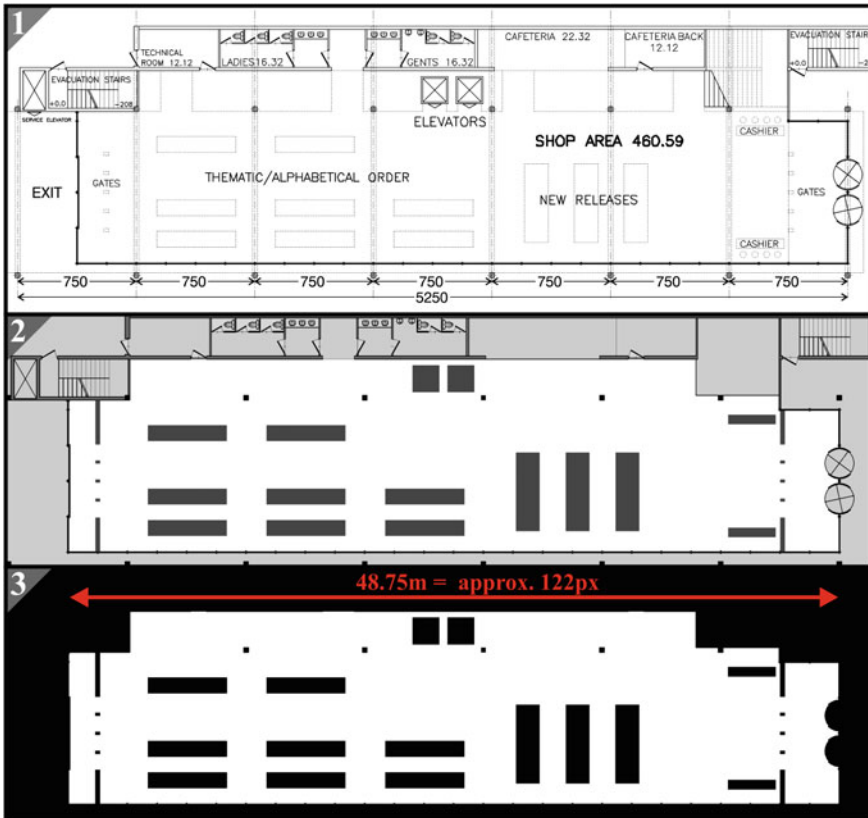
Fig. 5.1 1 The CAD-drafted layout of one floor of a retail shop. The surface areas and linear dimensions are given in: square meters and centimeters, respectively. 2 The pre-processed layout ready for export from CAD software. The “walkable” area is shown in white. 3 The bitmap of the CS environment ready for rescaling
