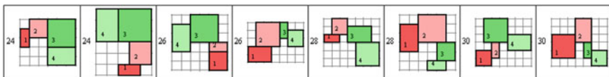
Fig. 1.22 Some examples of room configurations with external perimeters of different lengths. The perimeter lengths are shown on the left at each FL. Since the internal communication is not included in this computation, the corridor cells are hidden
